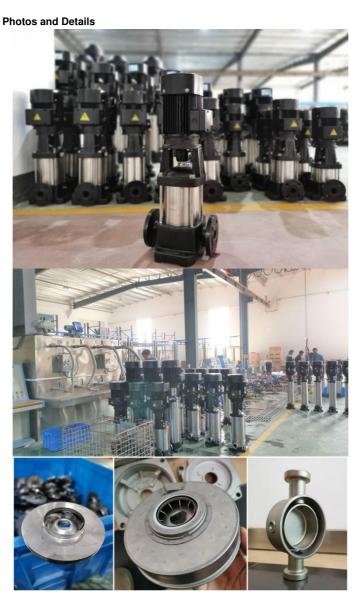
Design and Advantages Integrity pump set. Motor seated on pump, connected by couplings. Stainless steel impellers. Stamping-welded or precision-casted. Suction and discharge on the same level. High efficiency, energy-saving. Easy installation. Little space required. Easy maintenance. Sealing could be replaced as one piece. Model Explanation
